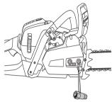
The chain is correctly tensioned when it does not sag from the underside of the bar, but can still be turned easily by hand. Hold up the bar tip and tighten the bar nuts with the combination spanner.
